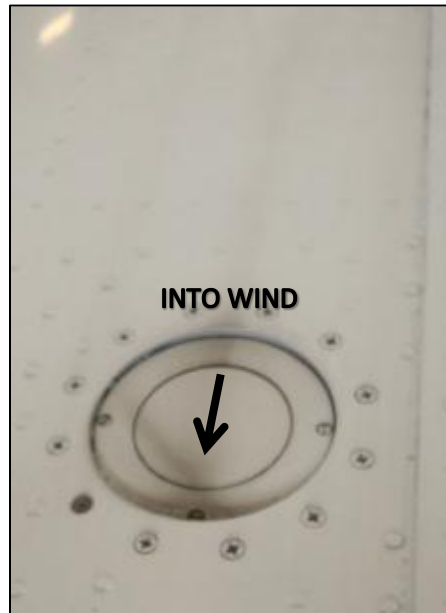
Photo 11 Smoke shutter fuselage cut-out from exemplar aircraft
