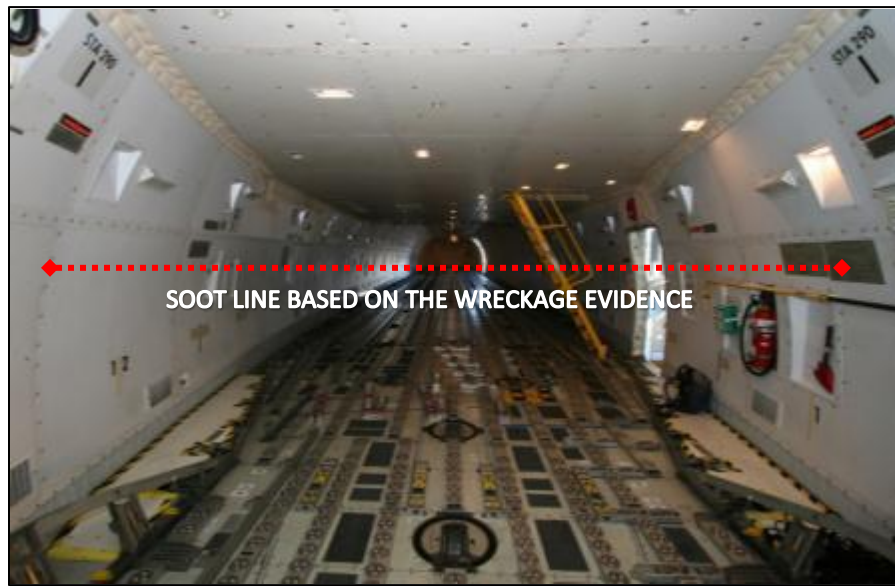
Photo 17 Exemplar interior showing stairs to the flight deck and a dotted line showing the level of the smoke layer
