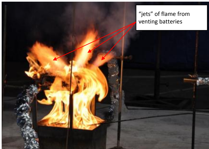
Figure 84: Box of lithium-ion batteries burning over propane burner exhibiting battery venting and electrolyte combustion
