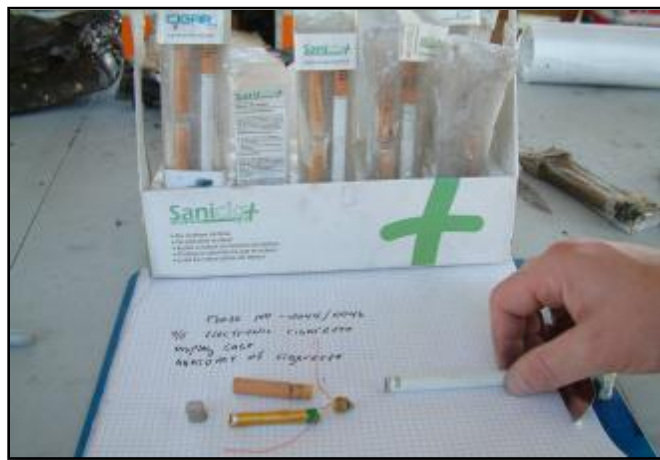
Electronic cigarettes containing lithium primary batteries 55
