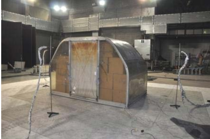
Figure 90: A2N type container with fuel load inside
