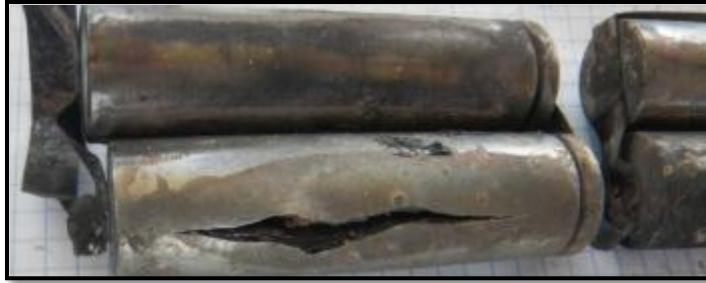
Fire damaged remains of battery pack with a fractured cell
