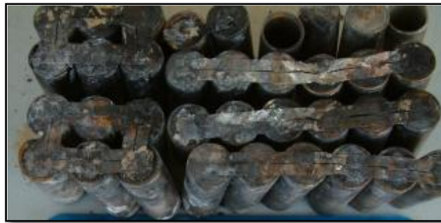
36-cell lithium-ion battery pack with multiple vented cells
