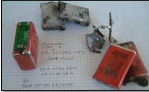
Intact and fire damaged Panasonic batteries (2-pack Li-ION set)[LH]/Mobile phones and batteries [RH]
