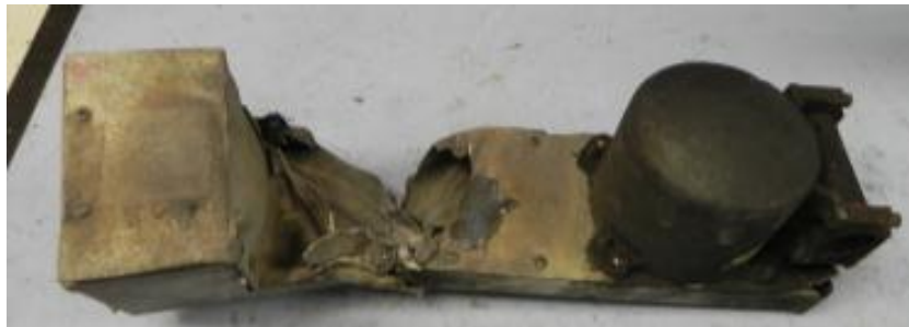
Picture 3 Damaged Flight Data Recorder in the Recovered condition
