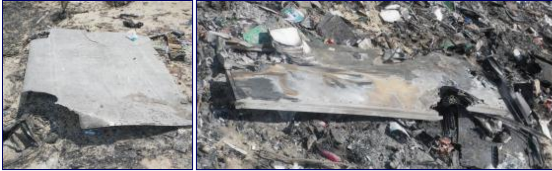
Photo 3 Cargo container base plate [LH] and cargo door [RH]
