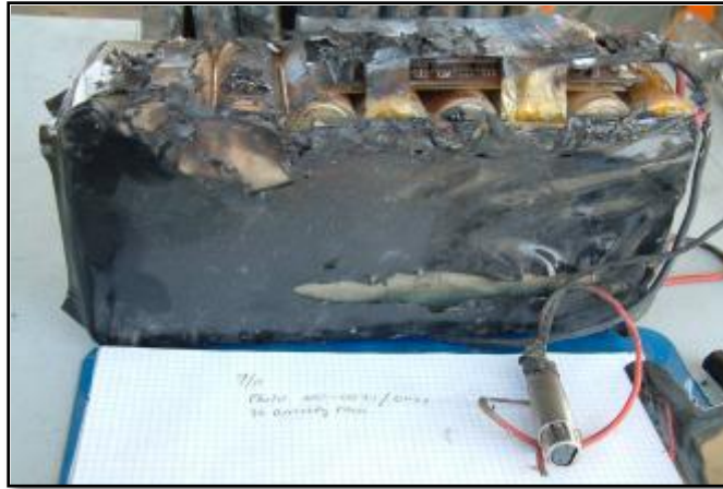
36-cell lithium-ion battery pack with thermal damage.
