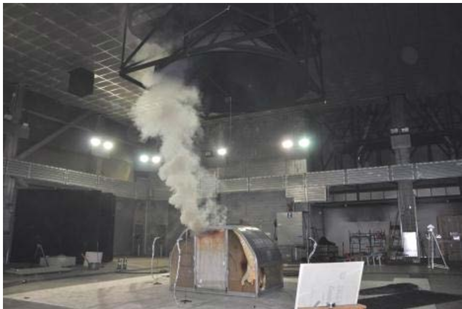
Figure 91: Smoke exiting above roll-up door on A2N type container
