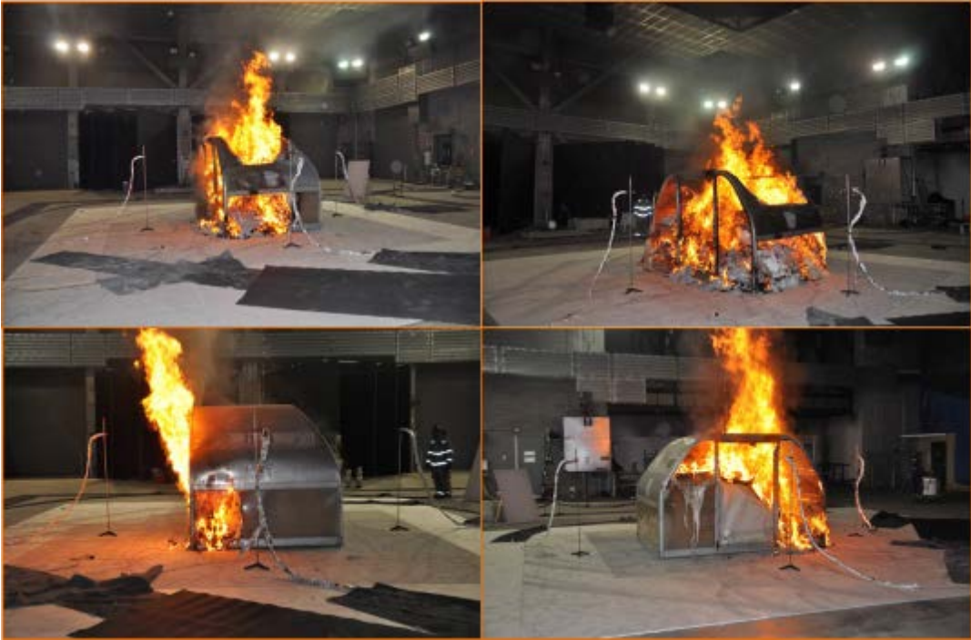
Figure 29 A2N Cargo Container Fully Developed Fire
