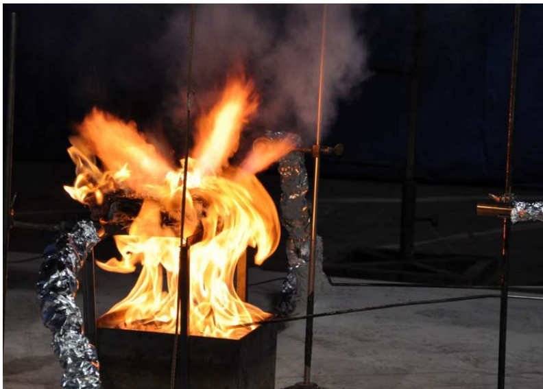
Photo 3- Venting of the electrolyte from a battery exposed to fire.
