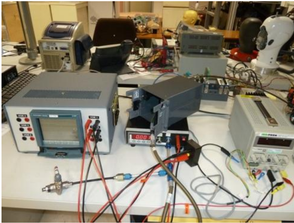
Figure 66 : Photo of MXP147-3 pressure switch actuation test set-up
